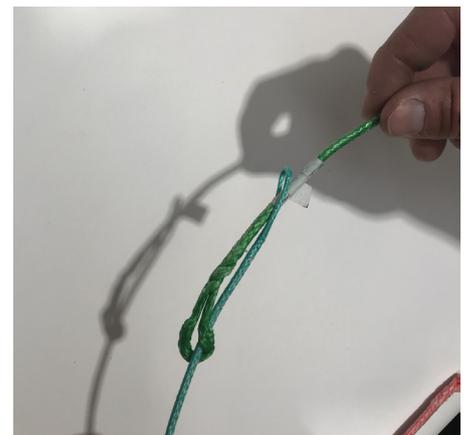
For North kites re-attach the Line Connectors\* to the ends of the new upper lines using the orientation outlined in Step 2.
