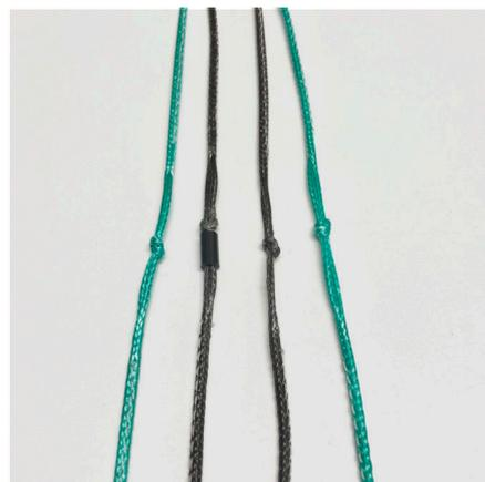
Attach the new upper lines at the length combination of your choice using the loop-to-loop connection at the line split. Ensure the lines are colour matched. Slide the line stopper back up towards the line split.
