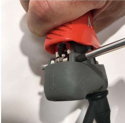
Locate the knurled locking pin that holds the release pin in place. The locking pin will be marked with a dot on one end. This is the end of the pin you will need to lightly tap to remove the release pin in order to access the small o-ring. Remove the Release Pin from inside the QR Body.
