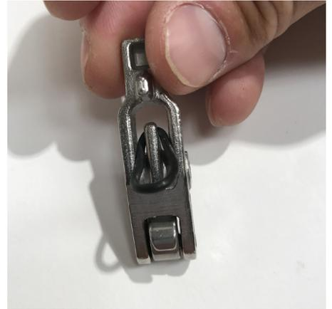
Remove the Release pin from the QR and locate the O-ring. Remove the old O-ring.
