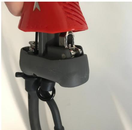
Re-install the release pin inside the QR Body by pushing the knurled locking pin back in place. Ensure each end of Locking Pin is flush with corresponding surfaces on the QR Body.
