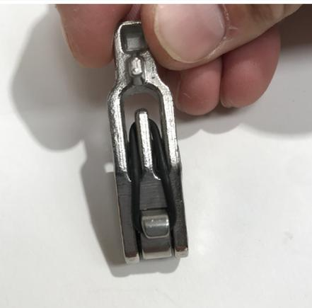
Take your new O-ring and hook it over the top of the release pin end and stretch it over the hook on the end of the cam part.
