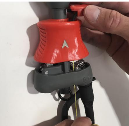
Thread both of the nylon/string lengths down inside the QR Handle and through the corresponding holes in the QR body.
