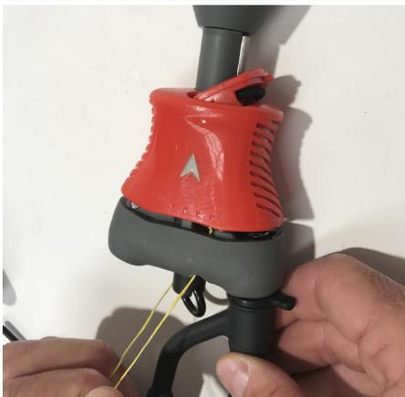
To fasten cap, insert small tab into the QR handle and push cap down into place.
