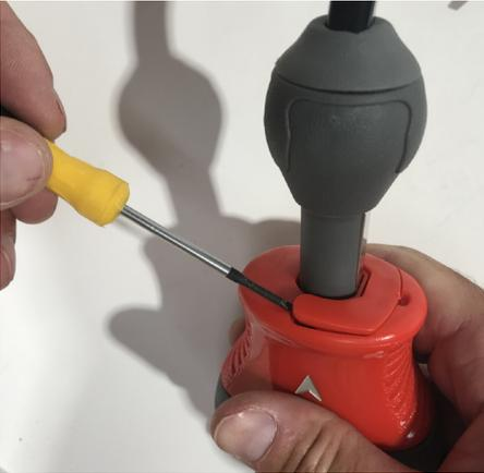
Open Quick Release handle. If old bungee cord and cap are still in place, cut the bungee to remove any remaining cord.
